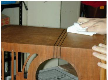
Fig13: Cleaning slop over from the groove edges.
