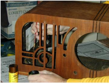
Fig12: Coloring edge of the speaker grill opening.
