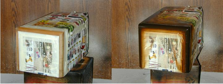
Fig14: Mask off the cabinet for major trim color- Fig15: Trim with 8 to 10 coats of tinted lacquer.
